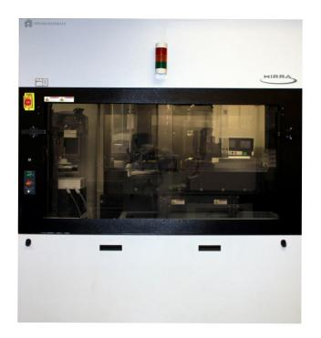
The Applied Materials Mirra CMP Tool is a Dry In - Wet Out (DI-WO) type of CMP machine which incorporates three polishing platens. The four wafer carriers are supported by a carousel transfer mechanism that moves the wafers through a one, two, or three step polishing process. It will process wafers from 150 to 200mm in diameter, and can be used for the planarization of thin films such as oxide, tungsten, and Polysilicon.
