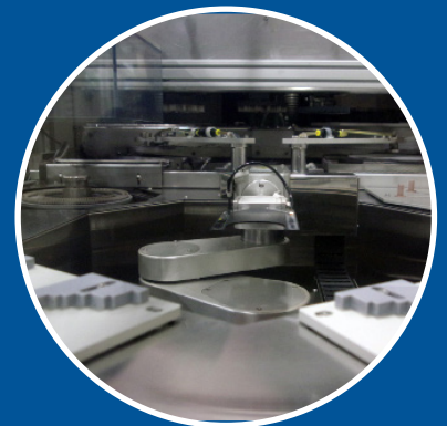
In-feed grinding w/wafer rotation
